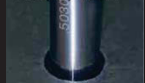
12 mm (1/2") hole without True Hole technology
